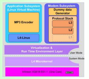
We estimate the virtualization overhead for various L4Linux applications and the performance of a real-time application under different system loads. In this setup, a native L4 hand-coded program which performs the data plane LTE protocol stack downlink functionality serves as realtime application at the modem subsystem .
