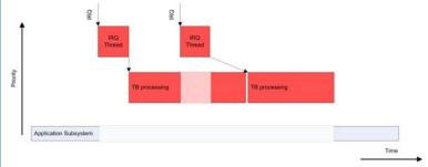
Depending on the data rate, the protocol stack consumes a maximum of approximately 25% of processing resources. The remaining resources can be used by the application subsystem, which causes cache contention and thereby affects the real-time application.
