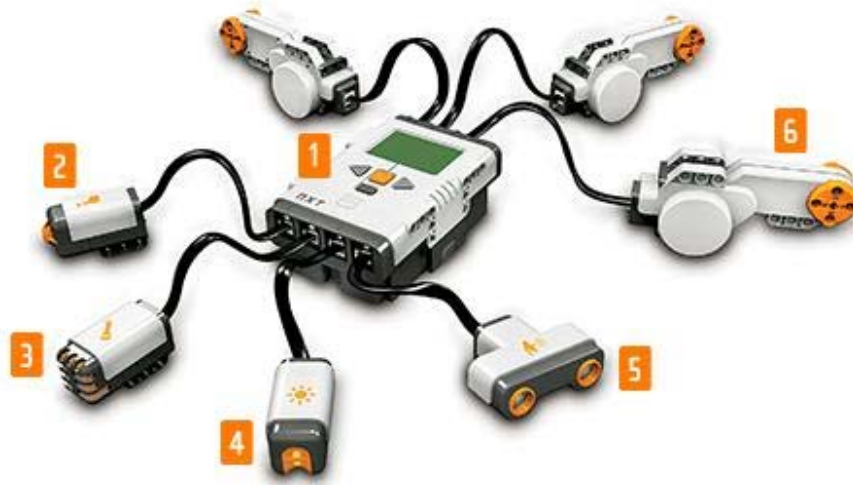
Fig. 8. The Lego Mindstorm NXT intelligent brick, actuators and sensors [20 - 22].
