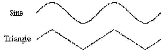
Fig. 2. Two common waveforms for delay variation (source: [3])
